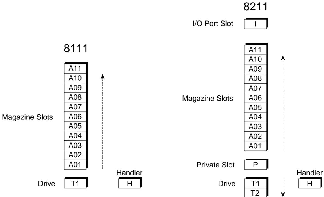
Figure 3-19 8111 and 8211 Cartridge Location Designators
