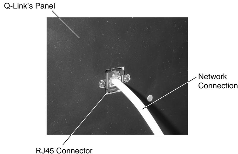
Figure 11-1 Detail of Network Connection Attached to Q-Link
