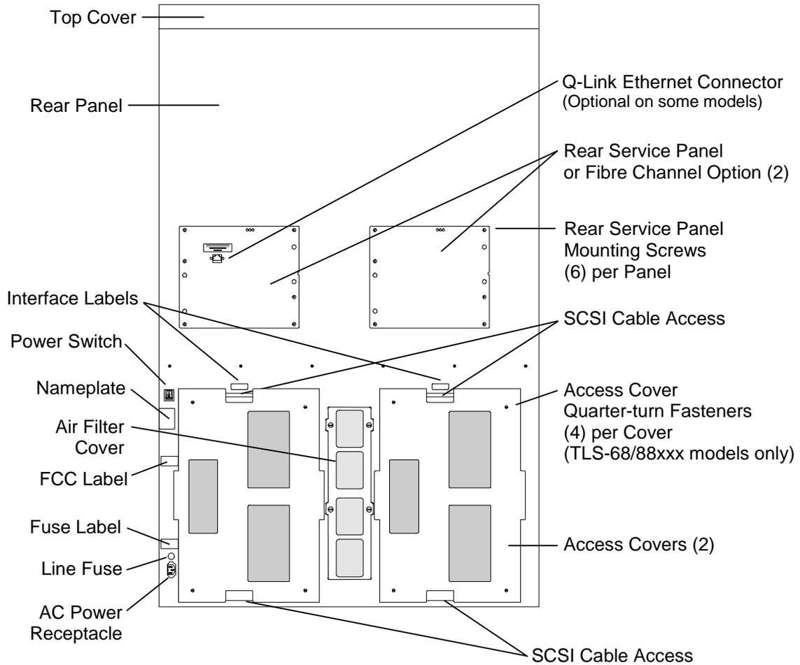
**Figure 3-7 58xxx, 68xxx and 88xxx Rear View with Access Covers Attached**
