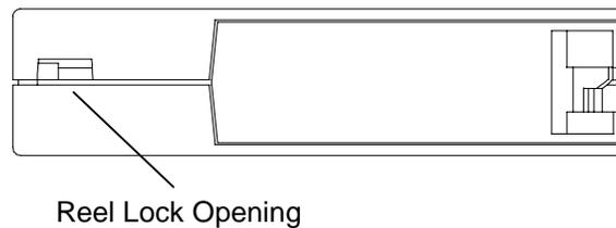
Figure 5-6 Location of Side Reel Lock Tab
