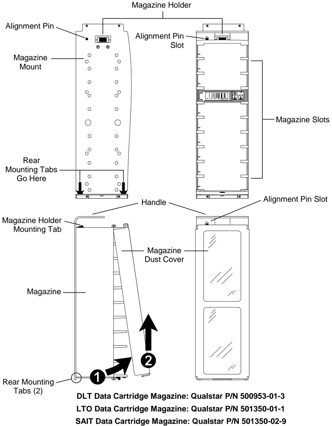
Figure 5-17 Magazine and Magazine Mount (DLT model shown)
