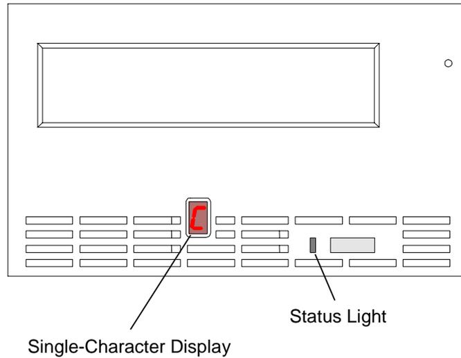
**Figure 12-9 IBM LTO Tape Drive – Front View**
