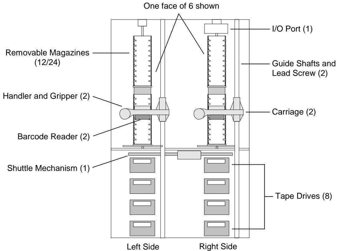
**Figure 3-10 TLS Major Internal Assemblies (Dual Bay Models)**
