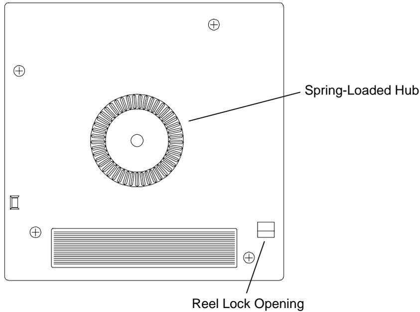
**Figure 5-7 Location of Bottom Reel Lock Tab**
