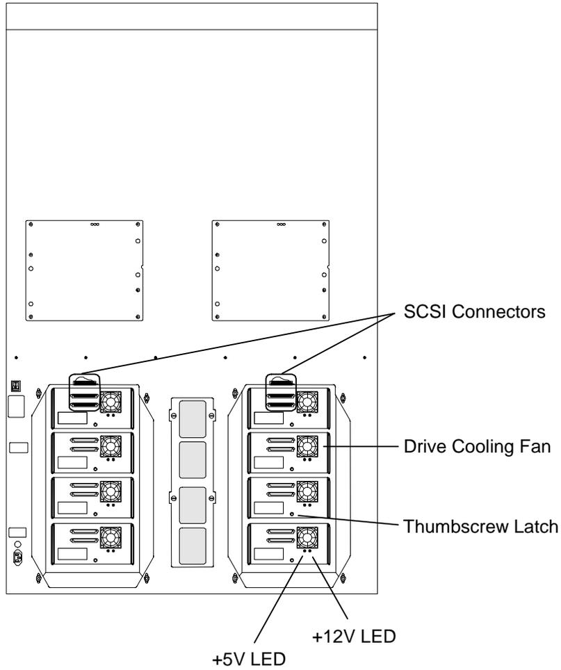
**Figure 3-8 58xxx, 68xxx and 88xxx Rear View with Access Covers Removed**
