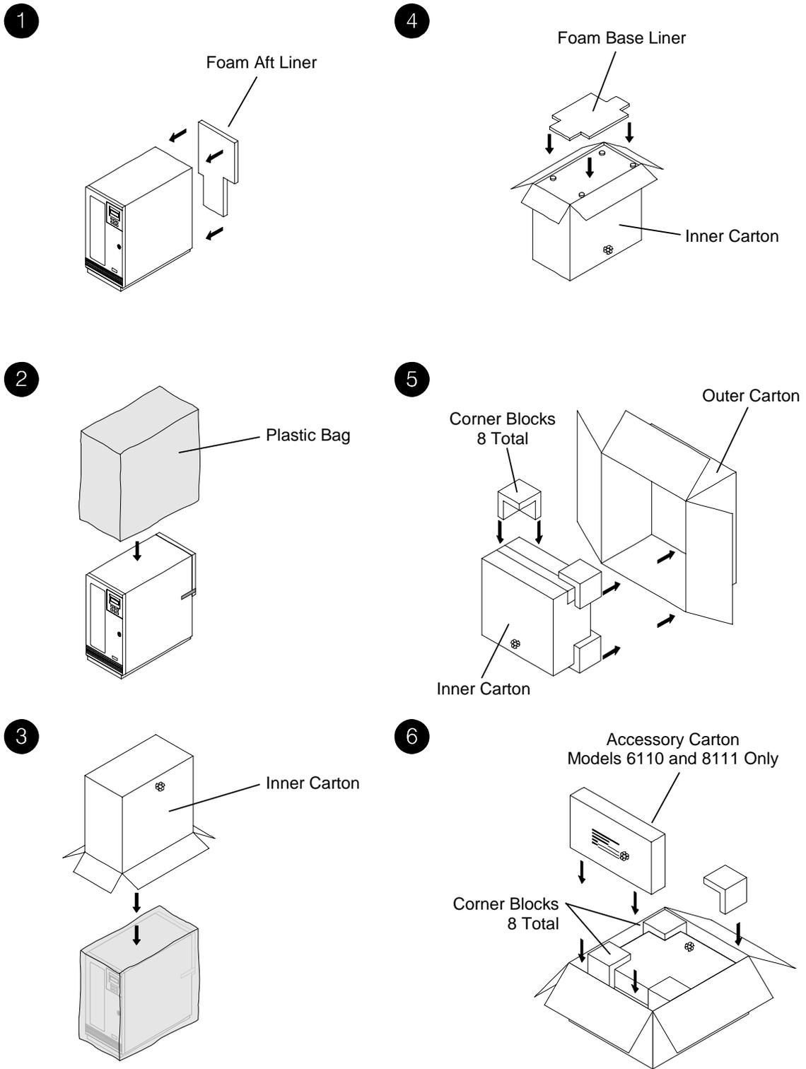
Figure 13-1 Repacking the TLS - Models 62xx and 82xx
