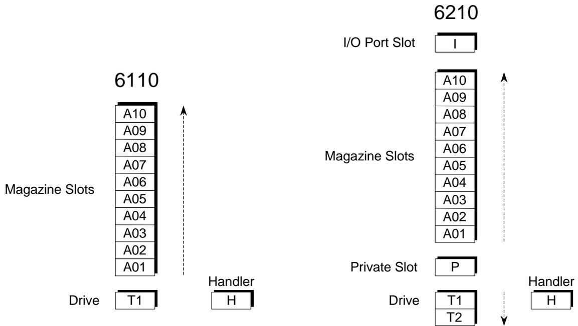
Figure 3-13 6110 and 6210 Cartridge Location Designators
