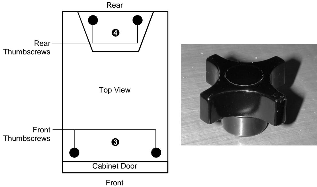
Figure 2-3 Cabinet Thumb Screws - Models 64xx and 84xx
