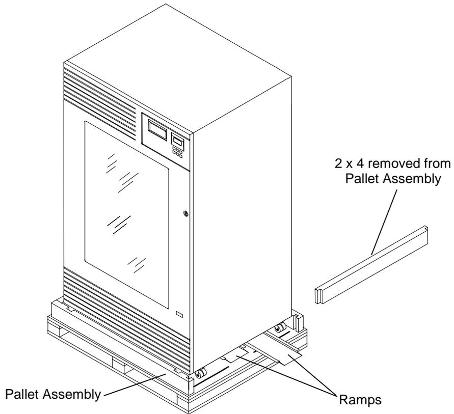
**Figure 2-8 2 x 4 Removed and Ramps Under the Library**
