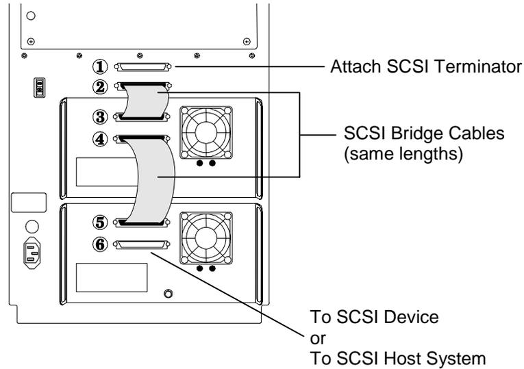
Figure 5-18 SCSI Basic Connection – Model 6220 Shown
