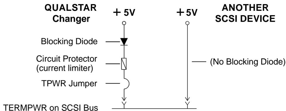
Figure 5-20 SCSI Termination Power Diagram
