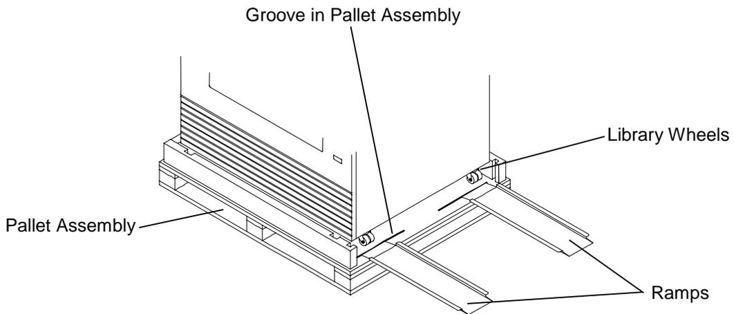
**Figure 2-9 Ramps Attached to the Pallet Assembly**
