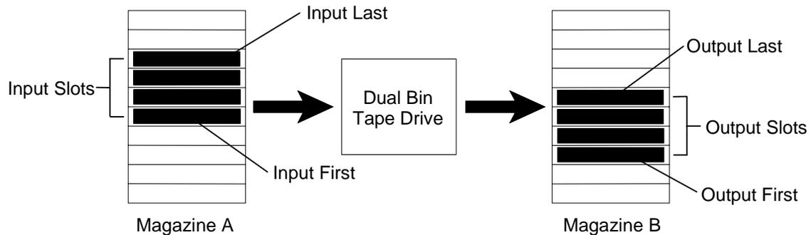
**Figure 10-2 Dual-Bin Configuration Example**
