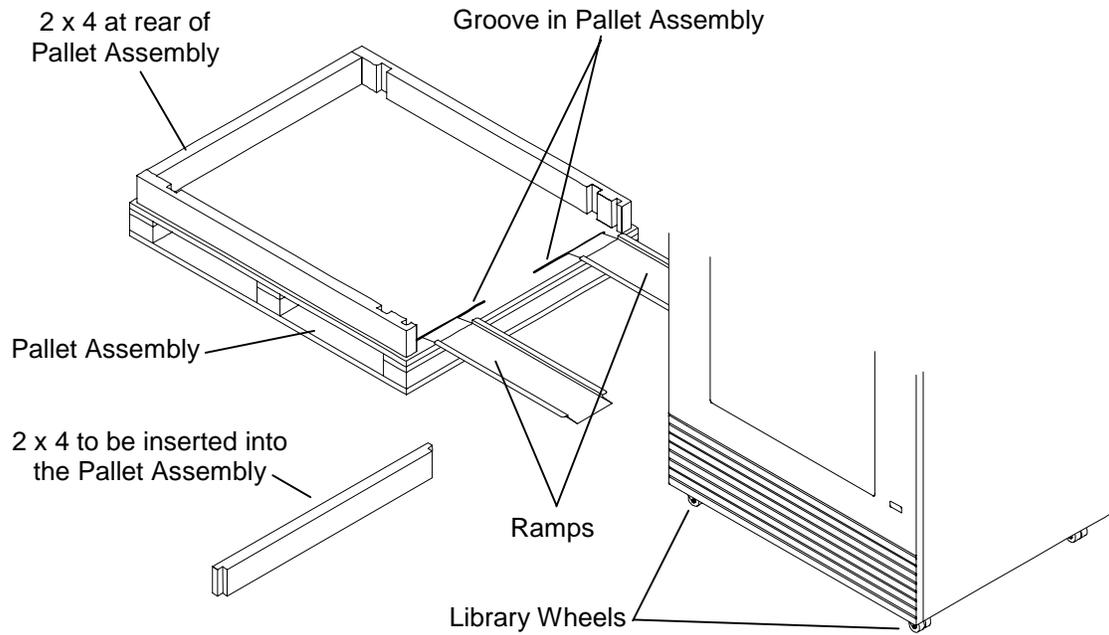
**Figure 13-4 Ramps Attached to the Pallet Assembly**
