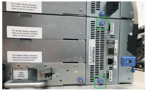
2. Using the thumbscrews, slowly remove the controller from the module.
