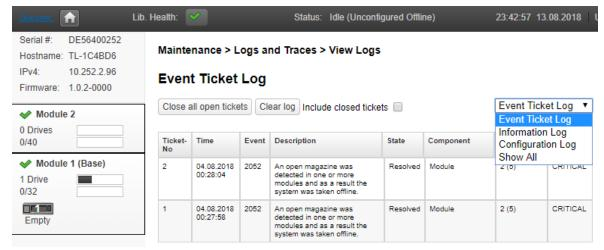
The log entries are displayed in order of most recent to oldest. The log entries contain a date and time code, event code, severity, component identifier and event details. The format for the date and time is: YY.MM.DD HH.MM.SS.ss.
