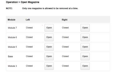
To unlock a magazine, click **Open** for the magazine. The library will release the lock. You can then pull the magazine out of the library to access the storage slots.
