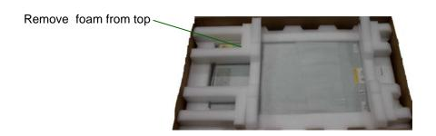
With assistance, lift the module out of the bottom foam nest, remove the wrapping from the module and then place the module on the work surface.
