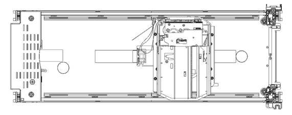
4. Lift the robotic assembly gently from the module and place it on top of the module on the right side (opposite the spooling mechanism) and slightly to the front. Take care not to damage the spooling cable.
