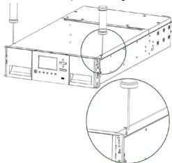
c. Lift the front end of the cover and pull gently forward to disengage from the pivot point at the unit center.
