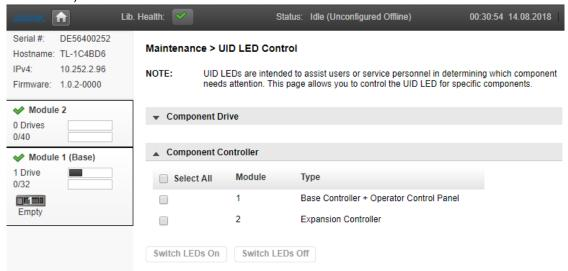
To use UID, navigate to Maintenance > UID LED Control.
