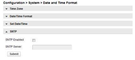
Check the SNTP checkbox. Enter the SNTP server IP address and click the Submit button.
