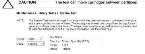
To run the system test, navigate to the **Maintenance > Library Tests > System Test** page, select the number of cycles and then click **Start Test**.
