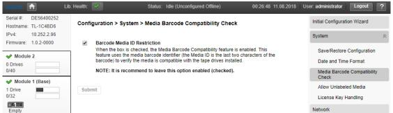
When **Barcode Media ID Restriction** is enabled, the library will only allow appropriate tape cartridges to be loaded into the appropriate tape drives. The barcode media ID is the last two characters of the barcode. For example, an LTO-6 labeled cartridge will not be allowed to move into an LTO-4 tape drive. When disabled, the library will move any tape to any tape drive. If the cartridge is incompatible with the tape drive, the library will display a message.
