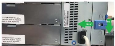
3. Go back to the front of the library, use a Phillips #2 screwdriver to loosen the captive screws fully on the module to be removed and slide the module out of the rack
