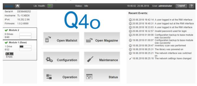
Click Open in the left or right magazine column within the module containing the magazine to be opened.
