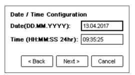
4. When finished with the date and time settings, select **Next>** and press **Enter** to switch where the Administrator OCP PIN can be changed.
