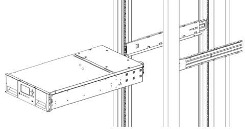
7. If you are installing multiple modules, verify that this module has been installed directly above or below its adjacent module and is contained within the correct 3U volume. The gap between modules must be less than 4 mm.
