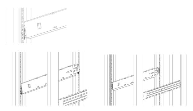
6. Place the library at the front of the rack on the support angles of the sliding rails and push it into the rack to the back stop.
