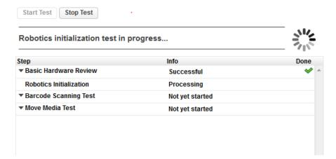
To run the Wellness test, navigate to the **Maintenance > Library Tests > Wellness Test** screen, and then click **Start Test**.
