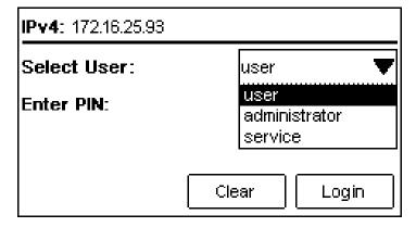
3. Then navigate to the Enter PIN field and enter the 4-digit PIN
