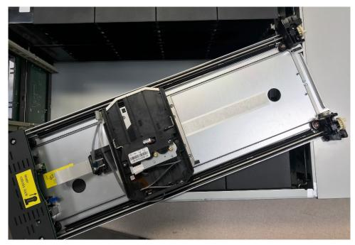
5. On the top of the robotic assembly where the spooling cable is attached, use a small flat head or Torx screwdriver driver to press and push the small latch that unlocks the spooling cable.
