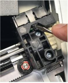
6. Lift the spooling cable from the robotic assembly and place it in its cradle at the top of the spooling mechanism.
